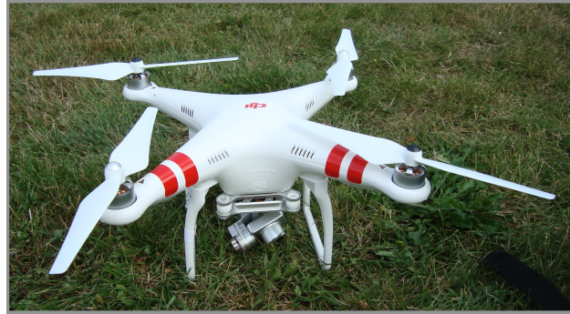
Figure 6.4: A Phantom quadcopter.
